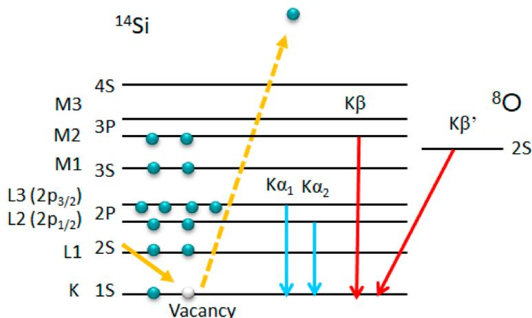
Fig. 5. Relationship between Si emission spectra and energy level diagram.
