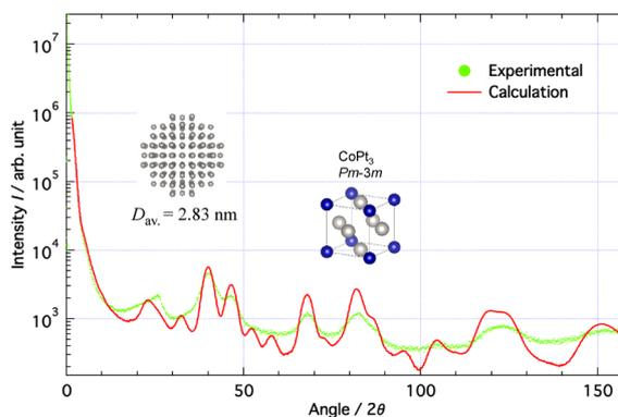
**Fig. 4.** Comparison of experimental and calculated profiles of small to wide-angle scattering/diffraction, assuming ideal atomic arrangement in the nanoparticle. The wider peak width of the experimental pattern means deformation of crystal structure of the nanoparticles.
