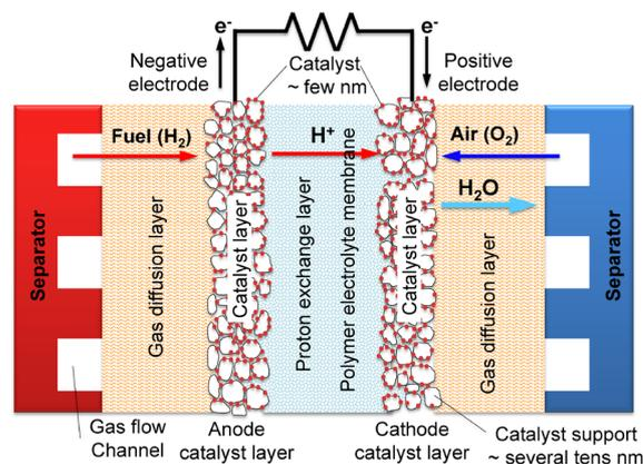
Fig. 1. Schematic view of fuel cell structure.
