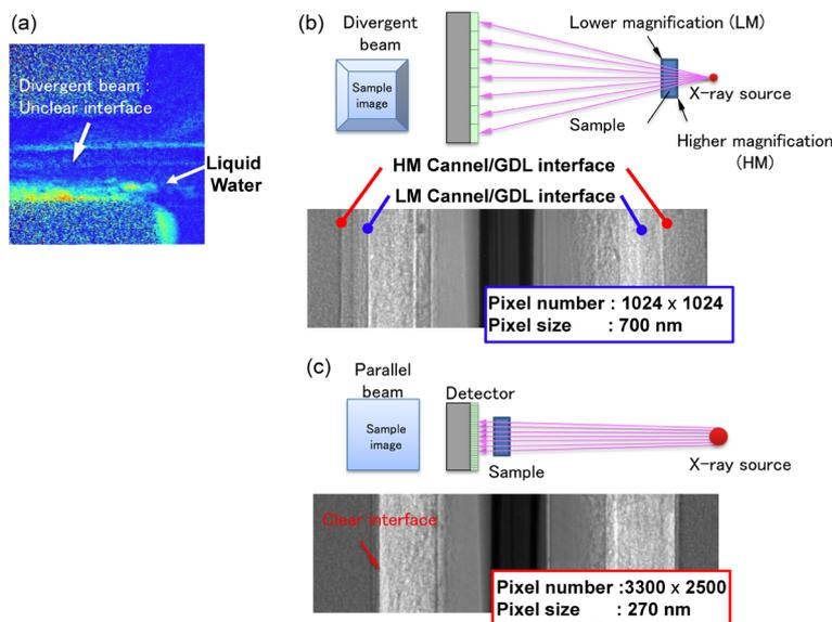
Fig. 9. Visualization of water flow in the fuel cell while generating electric power. (a) Water flow obtained by divergent X-ray beam projection. (b) Schematic and real image of divergent beam projection. Interfaces of each layer are not clear due to the different magnifications at the near and far side. (c) Schematic and real image of parallel beam projection and interface areas are clearly identified and investigated.
