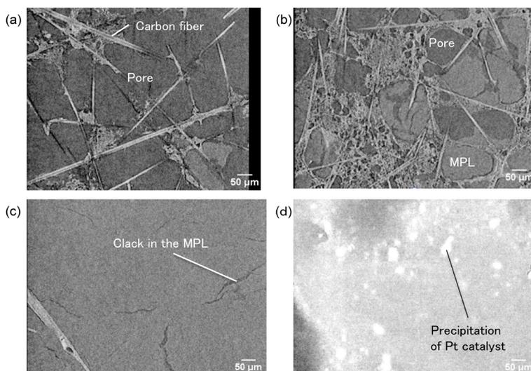
Fig. 8. Tomography images of (a) GDL, (b) GDL/MPL zone, (c) MPL, (d) catalyst layer.
