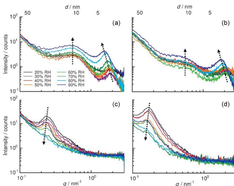
Fig. 5. Small angle scattering profiles for different kind of polymer membranes with changing humidity at 80°C<sup>(10)</sup>.
