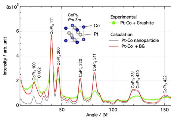
**Fig. 3.** Experimental and calculated X-ray diffraction patterns for Pt-Co nanoparticle with the size of 2.82 nm in diameter which is determined by small angle scattering shown in Fig. 2.
