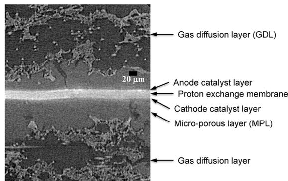
Fig. 6. Cross-section CT image for membrane electrode assembly (MEA). The structure shown in Fig. 1 is clearly recognized.
