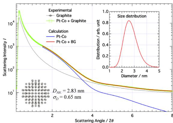
**Fig. 2.** Small angle scattering from catalyst particle on graphite support. Green line is the experimental and red line is the calculated profile. Inset is size distribution of the particle fitted to the experimental profile.
