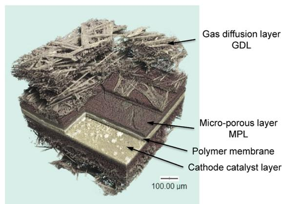
Fig. 7. Three-dimensional visualization of the MEA structure obtained by CT measurement.
