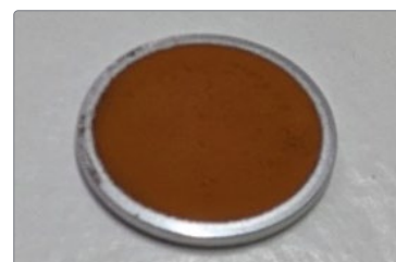
Figure 1: Pressure molding method sample preparation
