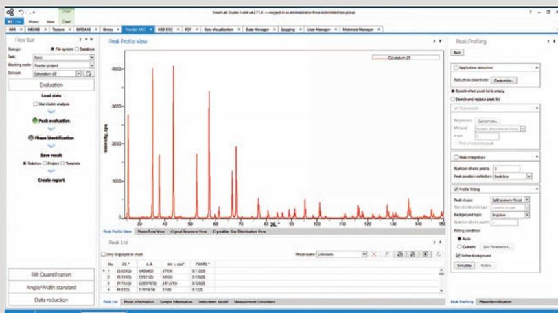
SmartLab Studio II is a new software package with a user-friendly GUI that integrates all measurements and analyses. Users can choose desired modules from various plugins, such as “XRD Measurement,” “Powder XRD,” and “Data Manager,” and operate them on a single platform with an improved analysis environment and operability.
