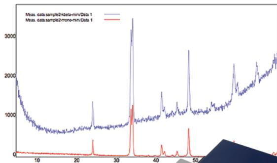
The red pattern illustrates background reduction when using the monochromator.
