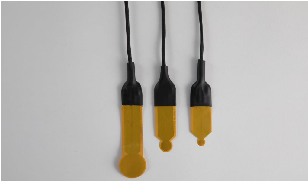
Figure 2. C-Therm FLEX Transient Plane Source Thermal Conductivity Sensor (Available in 6, 13 and 30 mm Size Options).
