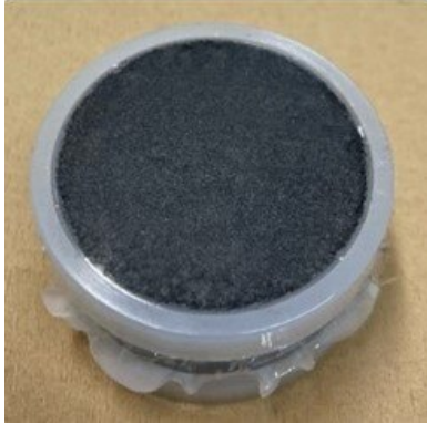
Figure 1: Sample preparation using loose powder method with commercially available graphite samples
