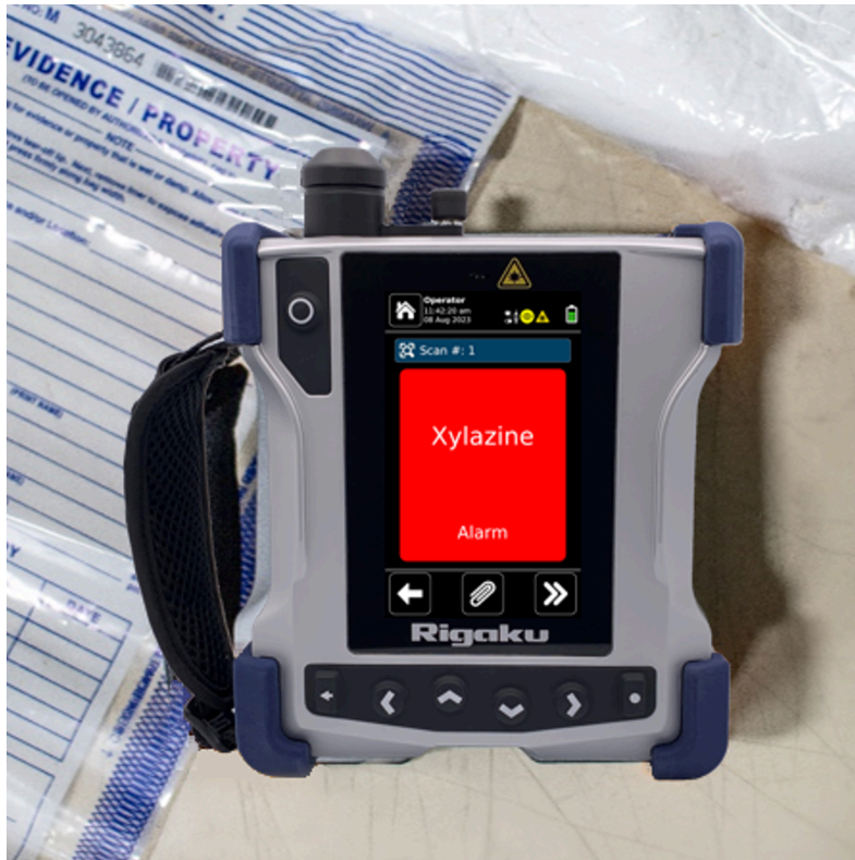
The Rigaku CQL Narc-ID 1064 nm Raman analyzer displaying a result for xylazine.
