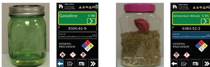
Figures 1-4. Analysis of gasoline through colored glass and analysis of ammonium nitrate through plastic container using a Rigaku CQL handheld analyzer.
