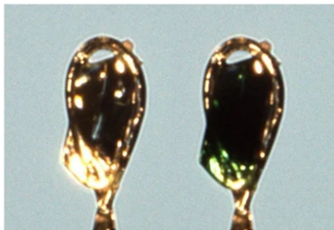
Figure 6: Pronounced discoloration of a ZnI 2 based crystalline sponge. Before measurement (left), after measurement (right)
