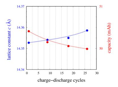
Lattice constant 'c' vs capacity with charge-discharge cycles Samples provided by Toray research center, Inc. 2. Fine in-situ observation of battery interior with XRM
