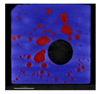
The void volume percentage within this solder connection was calculated to be 4.6%, also well below the maximum allowed value. The volume of each void was calculated. The figure below shows a volume histogram plot of the distribution of void volumes along with a 3D volume view, where both are color-coded according to volume size. Small voids are blue (<5e+6 cubic microns), large voids are red (~3.5e+7 cubic microns) and in between sizes are orange, yellow, and green.
