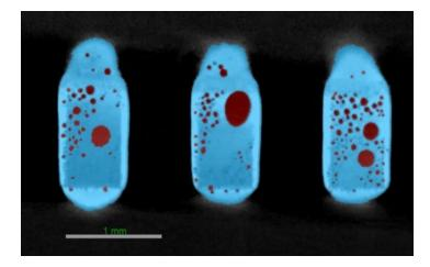
For example, this image shows voids in a 3D volume view, where total void volume within solders is calculated to be 7.7%. A more precise estimation of void volume can be evaluated using X-ray CT because these data allow us to analyze the void distribution in 3D rather than just in 2D. Large voids that overlap in a projected view can be separated and investigated individually, as demonstrated in the next section.
