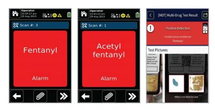
Result screens from the Rigaku CQL Narc-ID analyzer. The third image is an example of a result using QuickDetect Mode for non-visible sample analysis.
