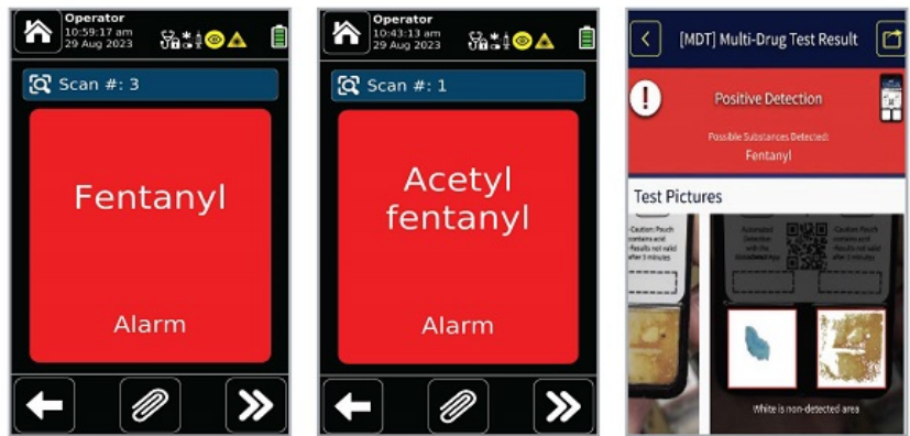
Result screens from the Rigaku CQL Narc-ID analyzer. The third image is an example of a result using QuickDetect Mode for non-visible sample analysis.
