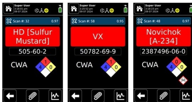
Figure 2. Result screens from the Rigaku CQL Max-ID for several CWAs using ThreatAlert scan mode.
