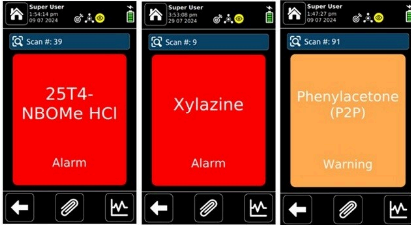
Figure 2: Examples of NPS materials detected by the Rigaku CQL Narc-ID, including 2C-derivatives, Xylazine, and drug precursor materials, such as phenylacetone (P2P).
