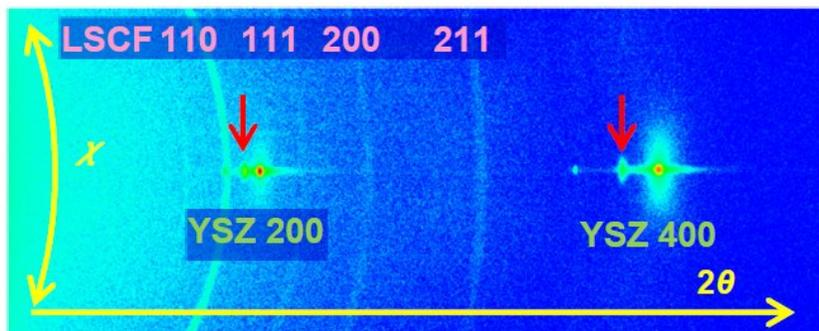
**Figure 2:** The 2D diffraction image for LSCF thin film using  $\text{CuK}\alpha_1$ .  $\downarrow$  were assumed to be diffraction peaks due to  $(\text{La}, \text{Zr})\text{O}$ .
