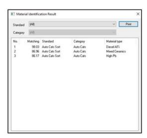
Identification of an aluminum titanate diesel cat.
