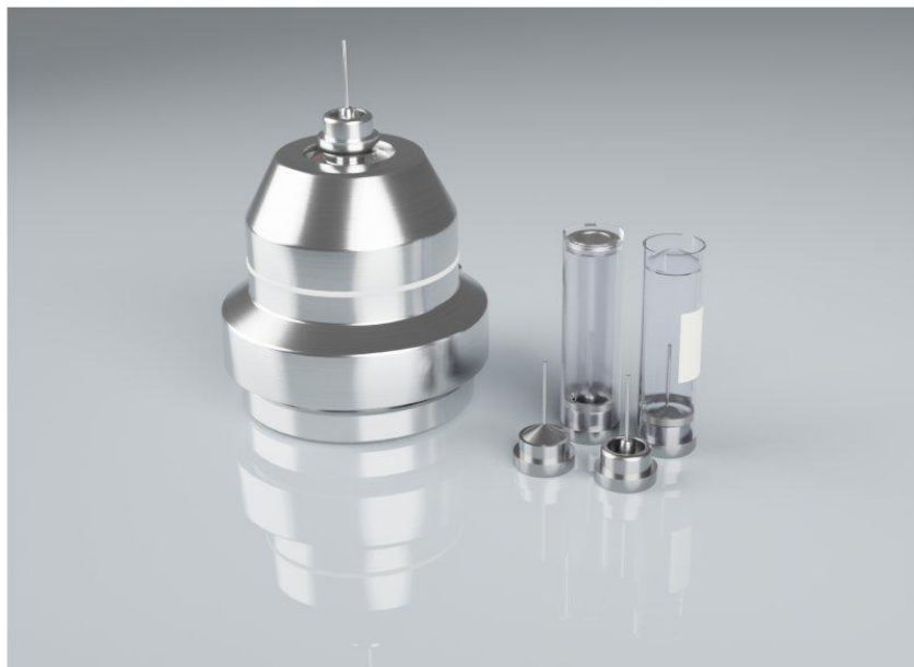
Figure 3: The IGH2 is a compact motorized goniometer head for automated crystal centering.
