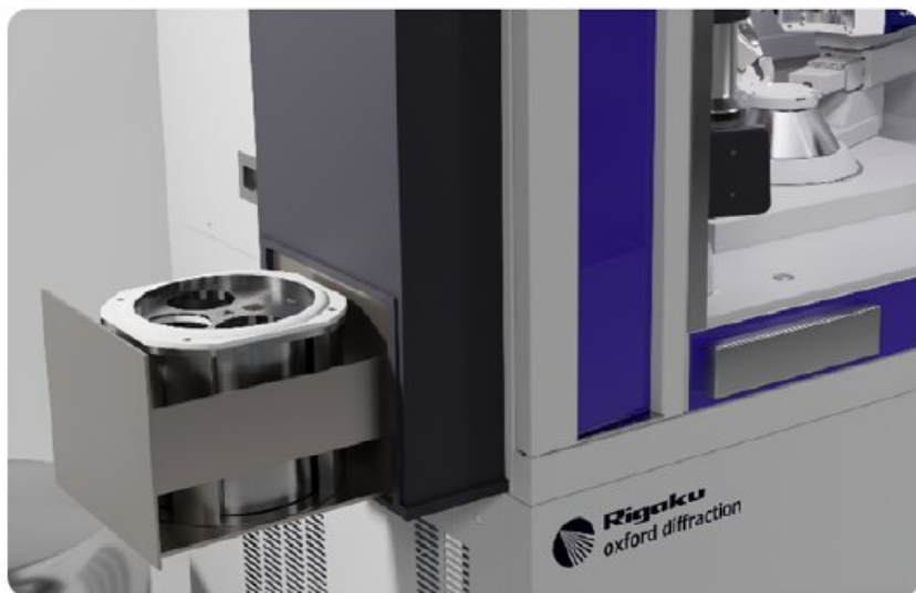
Figure 2: The XtaLAB Synergy Flow dewar opens by sliding out of the left side of the X-ray enclosure like a drawer.
