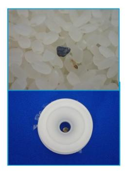
Measurement results using small spot point analysis indicated elemental composition consistent with a stone or a pebble, information that is helpful in tracing the origin of the source of contamination.
