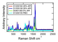
Different API loading in the capsule contents and the placebo are easily distinguished for these active compound formulations. This was demonstrated by measuring the contents of each capsule through plastic bags and adding each spectrum to Progeny's library. Figure 1 shows the spectra from these four samples.
