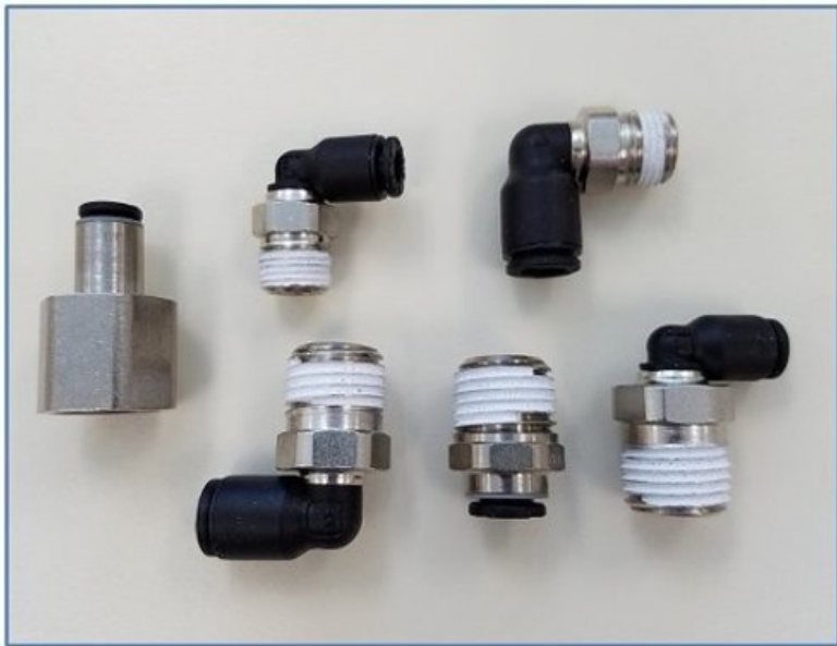
Typical tubing connectors with electroless PEN nickel coating.
