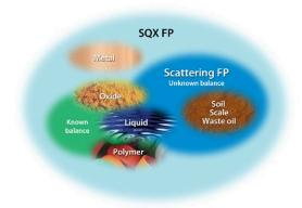
The Rigaku RPF-SQX software automatically deconvolutes spectral peaks and models the sample matrix and X-ray absorption and enhancement effects using fundamental XRF equations. The versatile RPF-SQX software is simple to use and offers many ways to craft a matrix model based on the specific material composition. This allows for semiquantitative analysis without the use of any reference standards, typically returning concentration results on the order of 15-20% relative.
