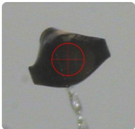
Figure 1: Catalase crystal. Crosshairs shows the beam position, and the circle is 0.2 mm in diameter.
