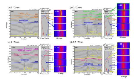
Figure 1: Results of simultaneous XRD-DSC measurement by different cooling rates
