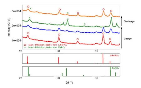
Figure 1: Phase changes in LiFePO<sub>4</sub> accompanying charge-discharge
