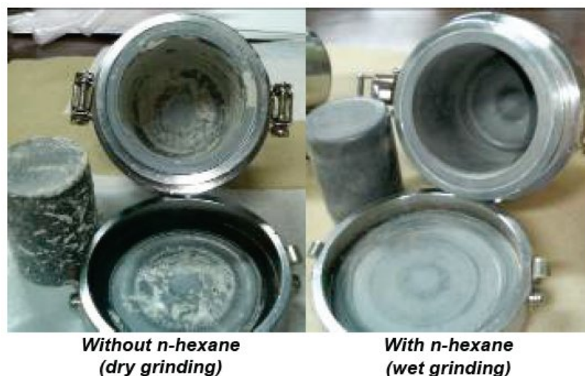
Figure 1: Comparison of the condition in the container after pulverizing
