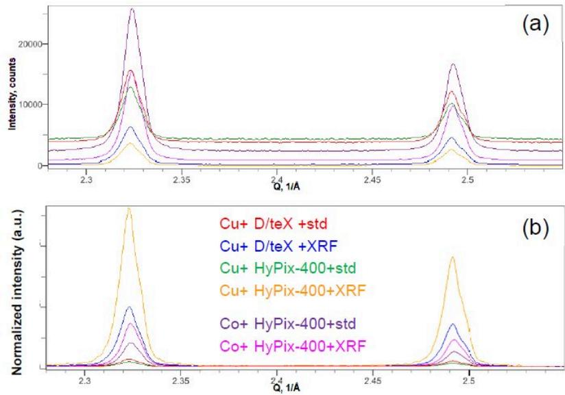
**Figure 1:** The observed diffraction profiles (a) and normalized profiles (b) of Fe<sub>2</sub>O<sub>3</sub> by Cu and Co sources, detector types, and their energy modes (Std: standard mode, XRF: X-ray fluorescence reduction mode ).
