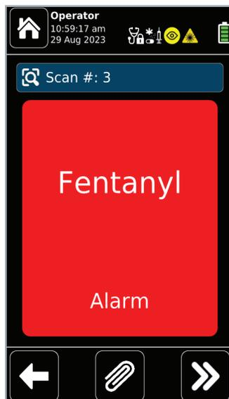
Examples of result screens from Rigaku CQL Series handheld 1064 nm Raman analyzers for chemical threat identification.
