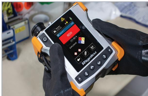
The Rigaku 1064 nm Raman analyzer displaying a result for RDX.
