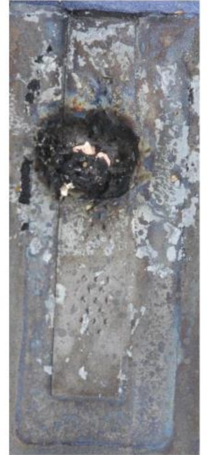
Negative Electrode Opposite Positive Tab
