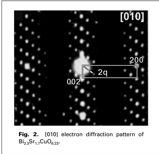
**Fig. 2.** [010] electron diffraction pattern of  $\text{Bi}_{2.3}\text{Sr}_{1.7}\text{CuO}_{6.23}$ .
