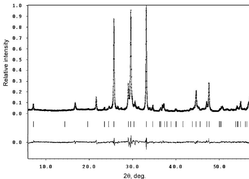
**Fig. 7.** Experimental, calculated and difference powder XRD patterns for  $\text{Bi}_{2.3}\text{Sr}_{1.7}\text{CuO}_{6.23}$ . Ticks mark the position of the main  $hk0$  reflections.
