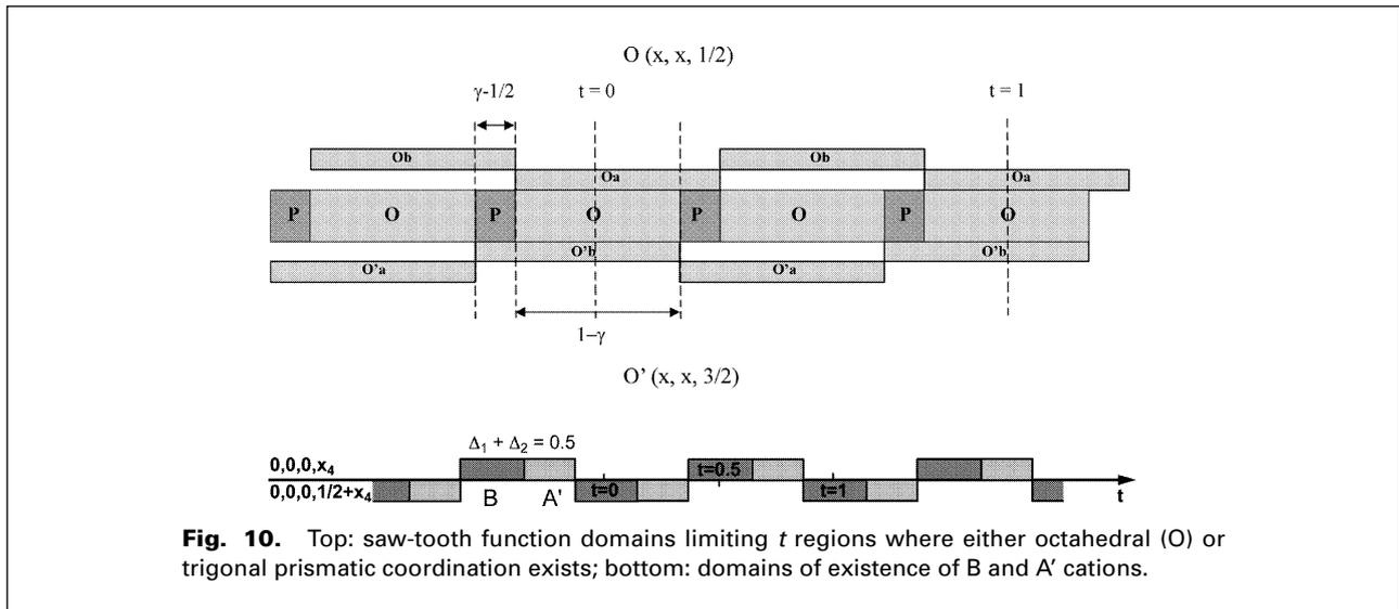
**Fig. 10.** Top: saw-tooth function domains limiting  $t$  regions where either octahedral (O) or trigonal prismatic coordination exists; bottom: domains of existence of B and A' cations.
