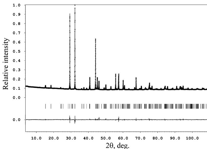
**Fig. 11.** Experimental, calculated and difference X-ray diffraction profiles for  $\text{Sr}_{1.32}\text{Mn}_{0.83}\text{Cu}_{0.17}\text{O}_3$ .
