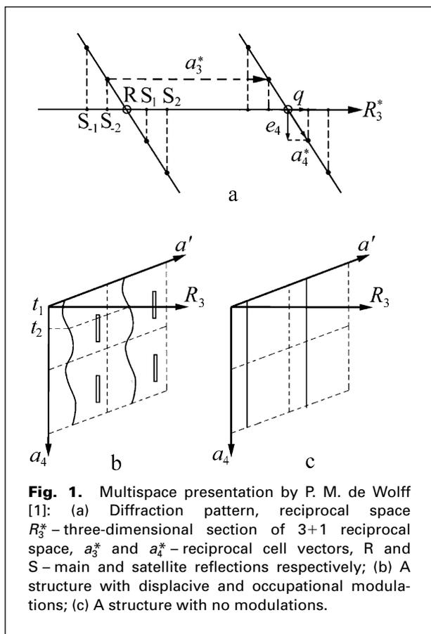
**Fig. 1.** Multispace presentation by P. M. de Wolff [1]: (a) Diffraction pattern, reciprocal space  $R_3^*$  – three-dimensional section of 3+1 reciprocal space,  $a_3^*$  and  $a_4^*$  – reciprocal cell vectors, R and S – main and satellite reflections respectively; (b) A structure with displacive and occupational modulations; (c) A structure with no modulations.
